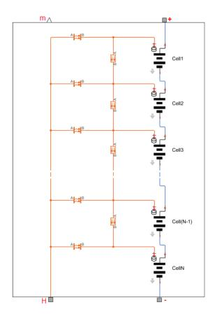
The composite component has two electrical nodes, p and n, and one thermal node, H:
