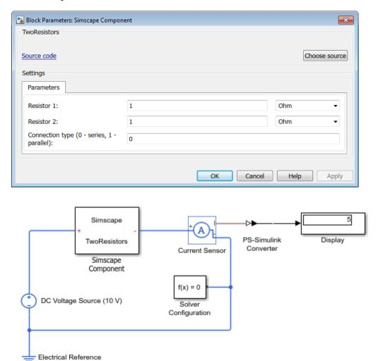
If you change the value of the **Connection type (0 - series, 1 - parallel)** parameter to 1, the resistors are connected in parallel, and the current is 20A.
