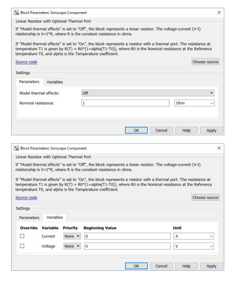
If the **Model thermal effects** parameter is set to **On**, the block represents a resistor with a thermal port, with temperature-dependent resistance. The block parameters, variables, ports, and the custom block icons change accordingly.
