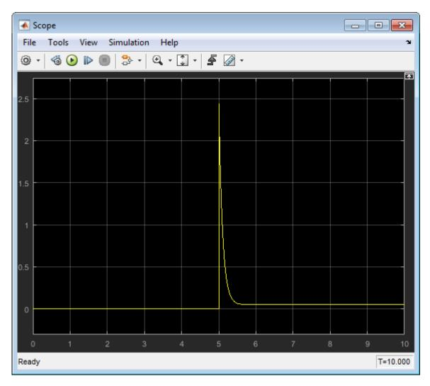
Simulation results show that, when the switch is flipped at t=5 seconds, the current delivered to the load is less than 2.5 A.
