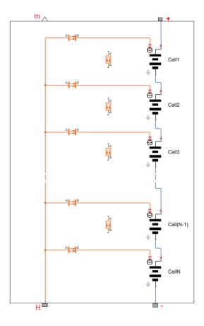
Finally, incorporate the thermal conduction elements by connecting node A to node H of the previous cell and node B to node H of the next cell:
