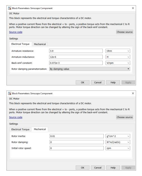
If you set the **Rotor damping parameterization** parameter to By no-load current, two additional parameters appear on the **Electrical Torque** tab, and the **Rotor damping** parameter on the **Mechanical** tab is hidden.
