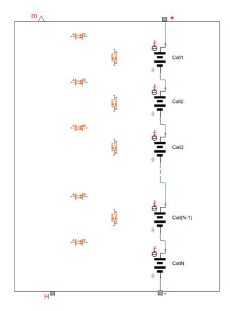
Use another for loop to connect thermal node H of each of the cells to node B of its respective convection component, and also to connect nodes A of all the convection components to thermal node H of the composite component:
